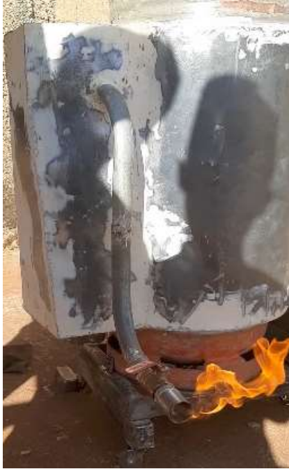
Figure 4: Production and flaring of syngas during gasification.
