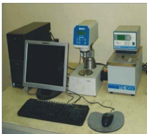
Figure 1: Rheometer set up for determination of rheological properties of yam flour
